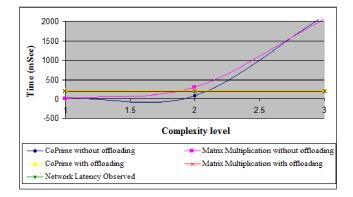
Fig. 2: Optimal Condition for Offloading
